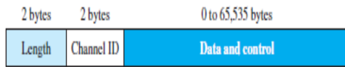
Fig.2.21 L2CAP data packet format
